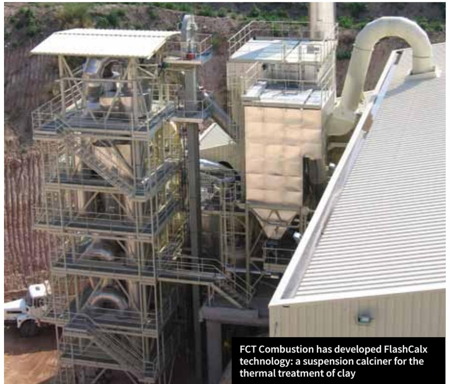
FCT Combustion has developed FlashCalx technology: a suspension calciner for the thermal treatment of clay
