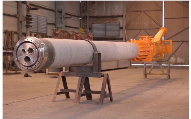
The Turbu-Jet AF burner for the CIMA Perlis plant.
